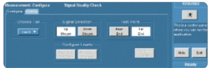
► Figure 2. TDSUSB2 compliance test package running on a TDS7404 DPO.
