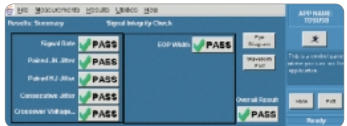
► Figure 3. Measurement results are automatically displayed using the TDSUSB2 compliance test package.
